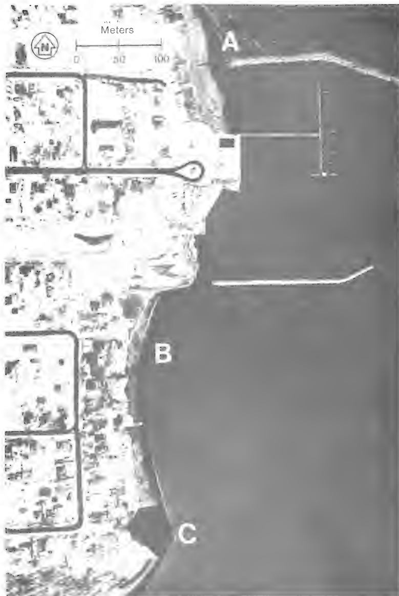
Figure 4. Lexington Harbor, 3 December 1980. A is the accretion area 2 months after removal of about 19,000 cubic meters of beach sediment; B is the part of the beach that received the 19,000 cubic meters of beach sediment from the accretion area; and C is the part of the feeder beach 2 months after receiving about 35,000 cubic meters of sediment from a nearby land borrow site.
